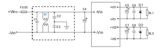
(1).C5,C7 is electrolytic capacitor, we advise to use High frequency low resistance electrolytic capacitor, the value is >80%, C6,C8 is for removing the high frequency noise, D1,D2 is TVS, it is for protecting the behind circuit.
